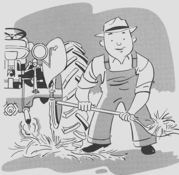
Keep Straw and Other Inflammable Material Away From Exhaust Pipe to Prevent Fire
